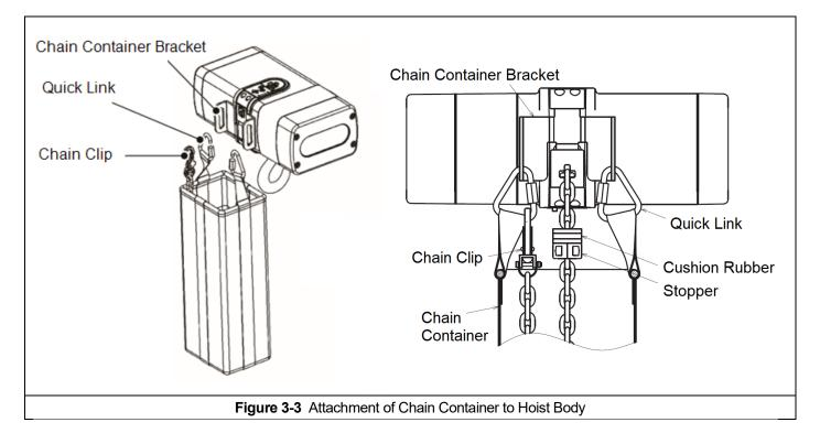
3.2.3 **A WARNING** Each chain container indicates the diameter and the maximum length of the load chain that can be stored in the container (refer to **Figure 3-4**). Be sure to check the label before installation. The amount of chain the container must hold is equal to the lift on the hoist. **Do** <u>NOT</u> use a chain container with a storage capacity less than the lift length on the hoist
