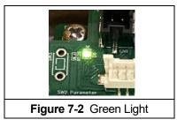
It remains turned on all the time during standby and assumes the following indication patterns during an emergency stop or operation (see **Figure 7-3**).
