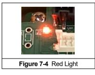
One complete error indication cycle is 14 seconds. A series of orange blinks displays in the first 4 seconds. The number of orange blinks signifies the "tens" place value of its error code. The red blinks display in the remaining 10 seconds. The number of red blinks signifies the "ones" place value of its error code. Reference the example in **Figure 7-5**.
