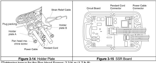
\*Tightening torque for the Pan Head Screws: 2.3 N-m (1.7 lb-ft)
