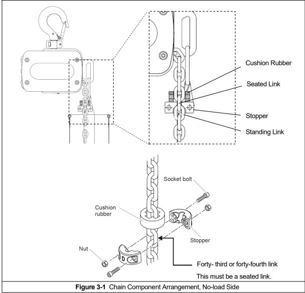
\*Tightening torque for the Stopper Bolt: 8.4 N-m (6.2 lb-ft)
