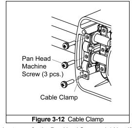
\*Tightening torque for the Pan Head Screws: 1.1 N-m (0.81 lb-ft)
