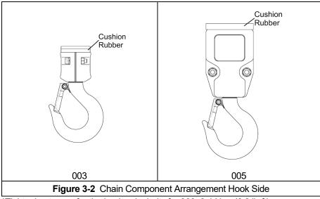
\*Tightening torque for the hook yoke bolts for 003: 8.4 N-m (6.2 lb-ft) \*Tightening torque for the hook yoke bolts for 005: 5.8 N-m (4.3 lb-ft)
