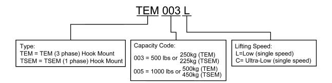
2.1.2 TEM and TSEM Models – KITO TEM series hoists are available in both three phase and single phase power. The TEM model is the 3 phase version and the TSEM model is the 1 phase version. Refer to Nameplate SP to verify the model by referencing the product code and voltage requirements. (See Figure 2-1)
