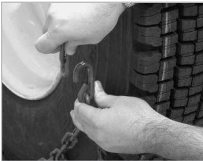
**4** Reach behind the tire and fasten the inside connector making sure it is as tight as possible. See the illustration below for a detailed look at this connection.
