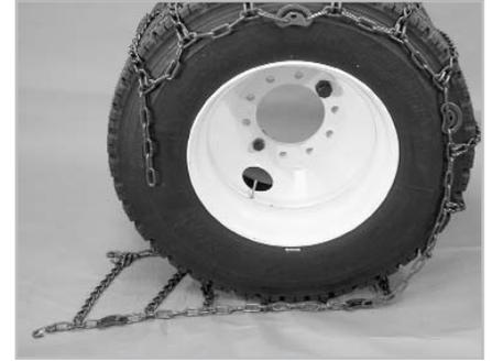
**3** Drive forward a few feet, far enough so that two or three of the cross chains pass under the tire.
