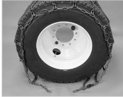
**2** Drape the chain over the tire, so that one cross chain is positioned at the point where the tire meets the ground. Again make sure the cross chain hooks are facing upward. Hooks that face down (towards the tire) will cause damage to the tire. "CAM" side adjusters should be on the outside of the tire.
