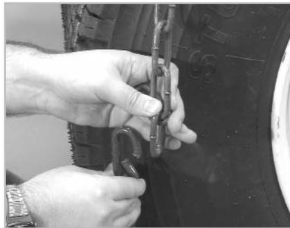
**5** Next fasten the outside fastener in the same manner, again making sure it is as tight as possible. Drive a short distance and retighten all fasteners. For best results, make sure fasteners are adjusted equally and as tight as possible.
