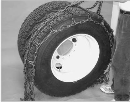
**1** Park vehicle on firm level ground, and turn off the engine. Set the parking brake. Lay the tire chains out flat on the ground, making sure there are no twists or tangles. Make sure the cross chain hooks are facing upward.
